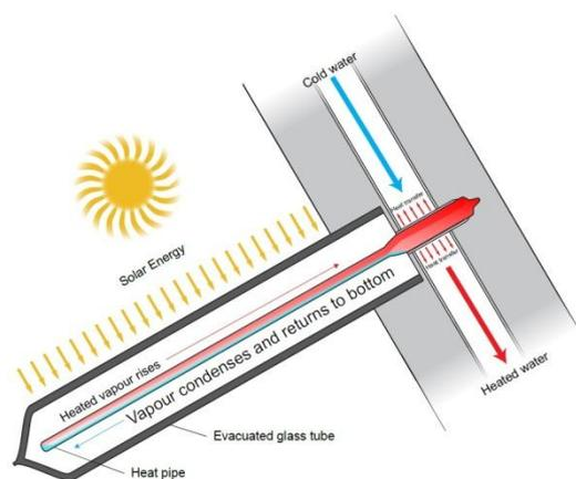
**Recommendation:** Where frost is a problem or where higher temperatures are required (eg in a commercial kitchen or laundry) then evacuated tubes are likely to be the best option.
